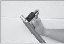
2. Twist the nub with the tool until the clamp breaks or loosens.
