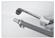
3. Remove the tool from the clamp, then remove the clamp from the pipe.
