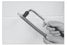
Slide the pinch clamp nub into the removal tool slot. If the nub is too large to fit into the tool, use the clamp tool to pinch the clamp one more time.
